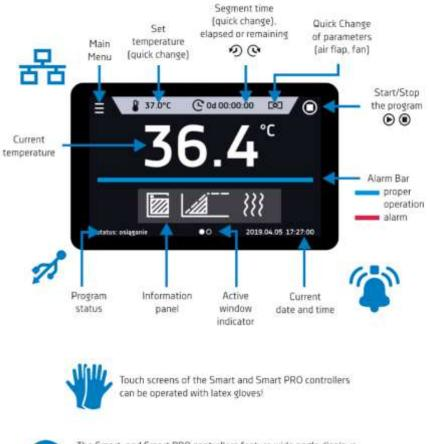
The Smart and Smart PRO controllers feature wide angle displays. You can see the screen clearly from any angle, regardless of the light intensity.
